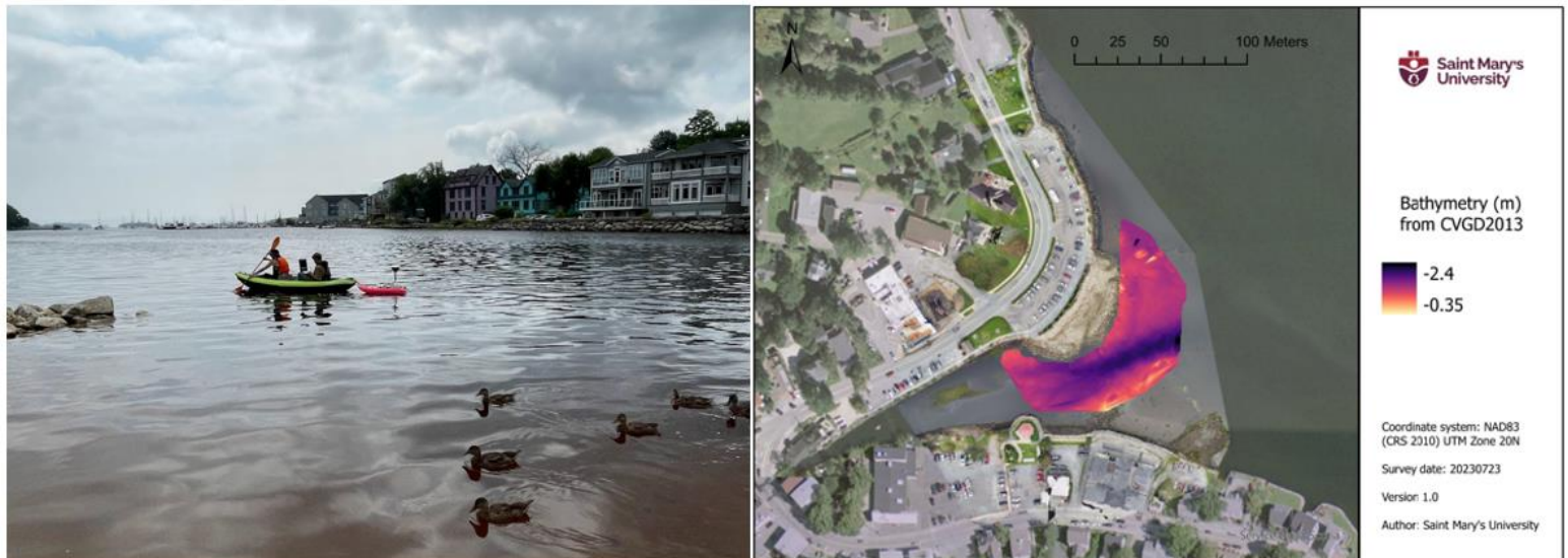
Figure 5: Left: Sontek M9 river surveyor being towed by TCA staff, picture taken by Leah Rudderham. Right: visualization of M9 survey results completed by Christian Hart.
